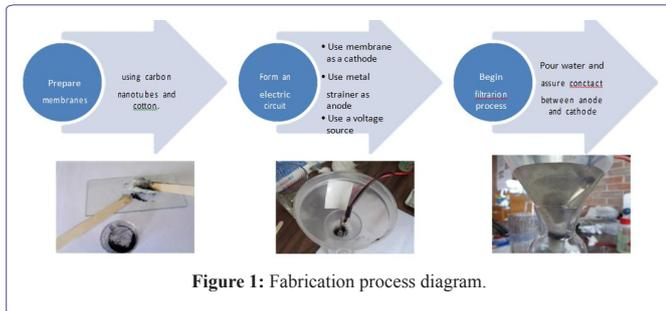
Figure 1: Fabrication process diagram.
