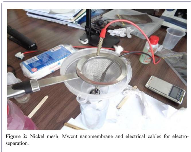
Figure 2: Nickel mesh, Mwcnt nanomembrane and electrical cables for electro-separation.
