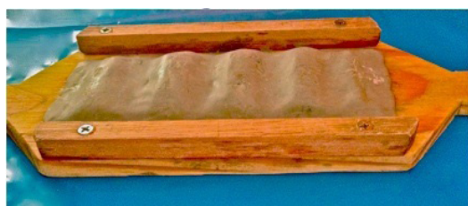
Figure 3A: Vertebral column phantom developed using Durepox™ resin, based on the anatomical information of Gocmen-Mas et al. [22].
