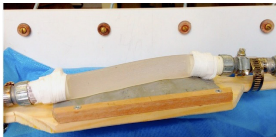
Figure 3B: Silicone aorta resting on the vertebral column phantom.
