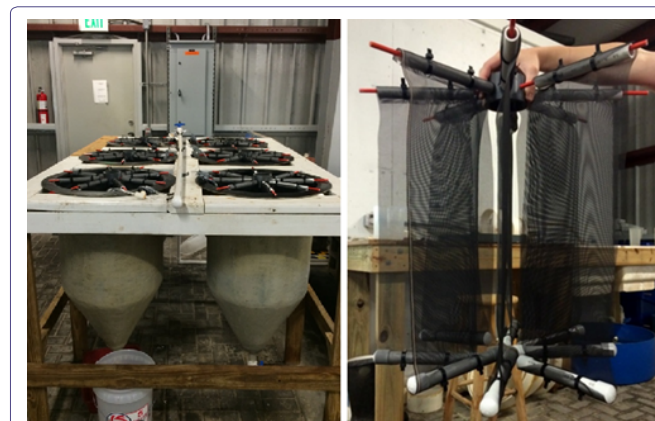
Figure 1: Amphipod culture system a) 60-L tanks and b) fiberglass screens.
