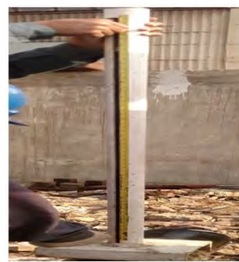
Figure 11: Shows impact test at fixed height of 1 meter.
