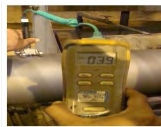
Figure 3: Temperature before shot blasting.
