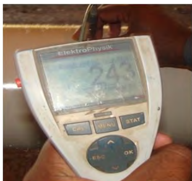
Figure 8: Shows epoxy cured film thickness 243 microns.
