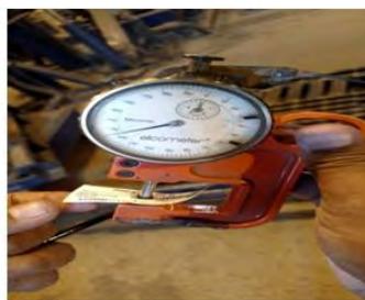
Figure 4: Shows shot blasted pipe surface profile.
