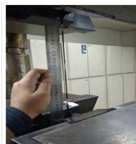
Figure 17: PE sheet Elongation Measurement
