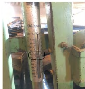
Figure 14: Shows peel adhesion value which is 240 N/cm.
