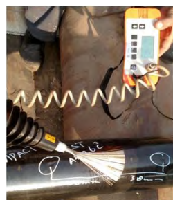
Figure 12: Holiday detection at 25 KV after impact test.
