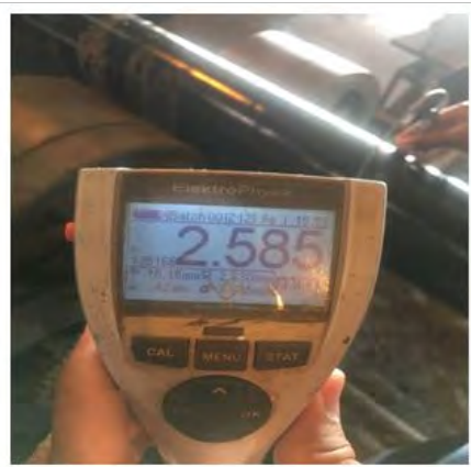
Figure 9: Shows 3 Layer thickness measured value 2.585 mm.
