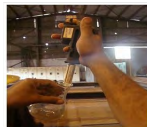
Figure 5: Shows chloride content test value after acid wash.
