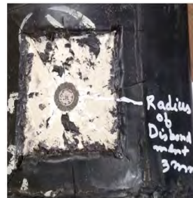
Figure 10: Cathodic disbondment test piece after test.
