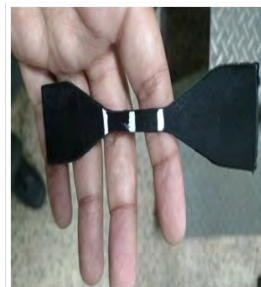
Figure 16: PE Sheet Elongation Test Specimen.
