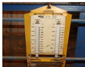
Figure 2: Showing dry bulb and wet bulb temperature.
