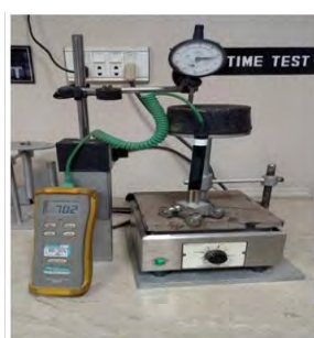
Figure 15: Indentation test of PE sheet @70°C.
