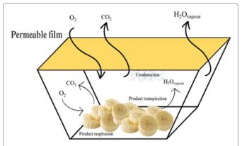
Figure 5: Schematic illustration of the interaction of packaging with modified atmosphere and your mechanism of favoring product shelf-life.
