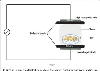
Figure 7: Schematic illustration of dielectric barrier discharge and your mechanism of operation.
