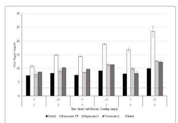
Figure 1: Enzymatic saccharification of untreated DDGS using different enzymes at three different enzyme dosages.
