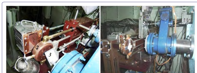
Figure 7: Experimental setup with labels showing the various components as labeled 1, 2, 3 and 4: 1 is the Faraday cup, 2 is the moveable target module and 3 is the luminofor for the beam spot size and position along with video TV control (left photo), and 3 is vibrating wire scanner module (right photo).
