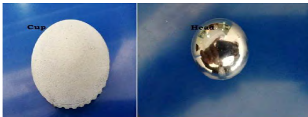
Figure 3: Hydroxy-apatite coated cup and metal head.
