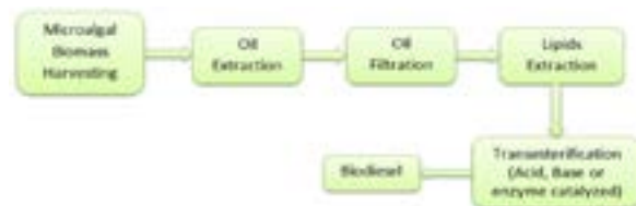
Figure 1: Microalgal biodiesel production pathway.
