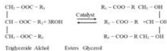
Figure 2: Chemistry of esterification.
